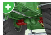
Weighing system , combinable with DPA (proportional flow).
