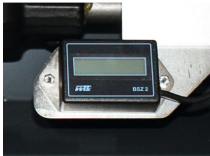
Operating hours counter
